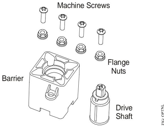
**Figure 16: Optional M9000-561 Thermal Barrier**
