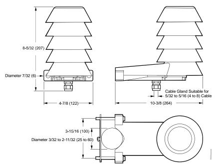
Figure 1: Hx-68P3 Series Outside Humidity and Temperature Transmitter Dimensions, in. (mm)
