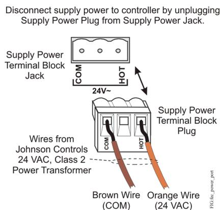
**Note:** The supply power wire colors may be different on transformers from other manufacturers. Refer to the transformer manufacturer's instructions and the project installation drawings for wiring details.
