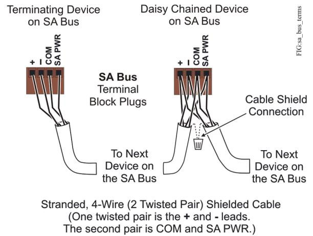
**Note:** The SA PWR terminal supplies 15 VDC. The SA PWR terminal can be used to connect (daisy chain) the 15 VDC power leads on the SA bus.
