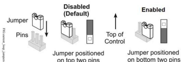
Setting the current loop jumper to the Enabled position (Figure 13) connects an internal 100 ohm resistor across the UI terminals, which maintains the 4–20 mA current loop circuit even when power to the controller is interrupted or off.
