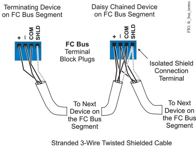
**Note:** The FC bus Shield (SHLD) terminal is isolated and can be used to connect (daisy chain) the shields for FC bus wiring.
