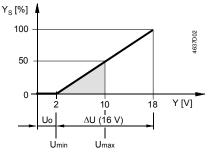
Max. positioning range Ysmax = 100 % (60 mm) 50 % (30 mm) 2 V Span range Ys = Offset Uo = Span ∆U = 16 V
